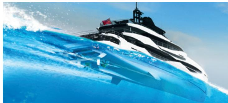
Some of the technical details of the Sunseeker 161 made of aluminium in partnership with Icon yacht have been released. The pleasure ship will be capable of speeds in excess of **22 knots** thanks to the sophisticated shape of its Fast Displacement Hull, FDHF, designed by the Dutch engineering studio **Van Oossanen Naval Architects**.
